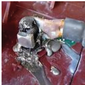
Figure 4- melted battery terminal
