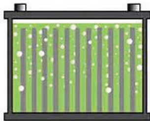
Figure 2- without acid stratification
